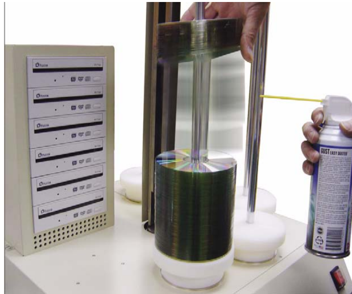
Figure 1-1 Using Canned Air to Reduce Static
